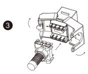
Position the termination cap on the keystone IDCs, in the correct orientation.
