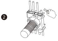
Insert the cable through the termination cap, untwist the four pairs and fan out. Following the colour code on the cap, insert the wires into their designated slots. Double check the wires are in the correct positions and then trim off the excess.
