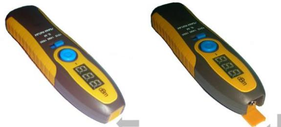
Lift the Dust Cap for access to the connector
